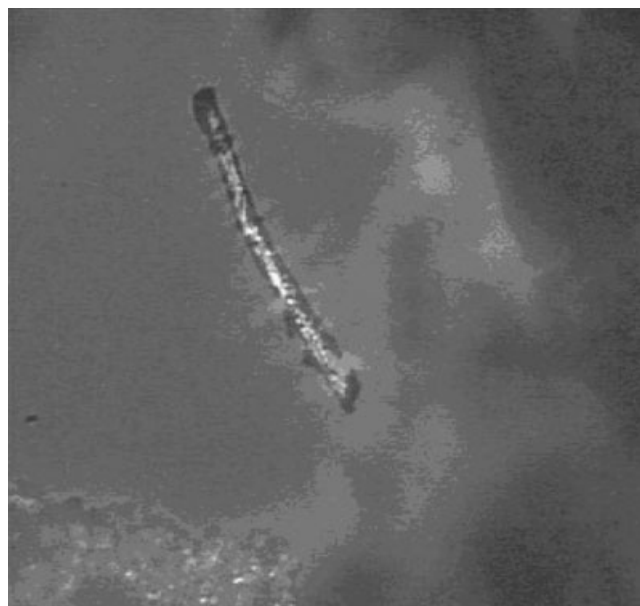
Figure 8 Optical texture of polymer P-4 at 209^\circ\text{C} on heating.
